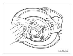
8) Remove any rust or dirt from the wheel bolts, mounting surfaces and spare wheel.
